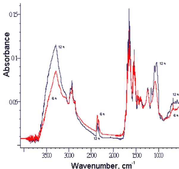
**Fig. 5.** Effect of the growth time on the FT-IR spectra from whole bacterial cells grown in a glucose culture medium. Red=6 hrs, blue=12 hrs.
