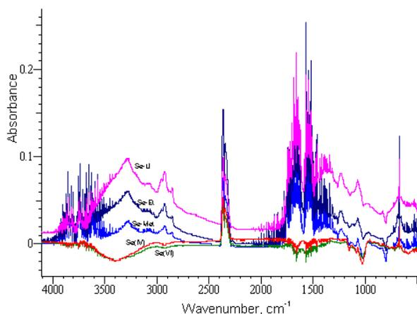
**Fig. 1.** Difference FT-IR spectra. They were obtained from the FT-IR spectra from whole bacterial cells grown in a glucose culture medium together with the analytes (50 ng ml<sup>-1</sup>) minus the FT-IR spectrum from whole bacterial cells grown in a glucose culture medium. From top to bottom at 3100 cm<sup>-1</sup>: Se-U (violet), Se-Et (dark blue), Se-Met (light blue), Se(IV) (red), Se(VI) (green).
