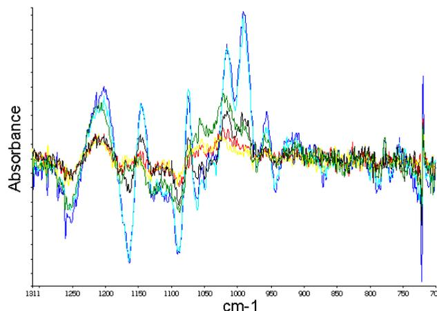
**Fig. 3.** First derivative FT-IR spectra derived from whole bacterial cells grown in a glucose culture medium (black) and glucose together with 50 ng ml<sup>-1</sup> Se-Met (dark blue), Se-Et (blue), Se-U (green), Se(IV) (red), and Se(VI) (yellow), over the same time.
