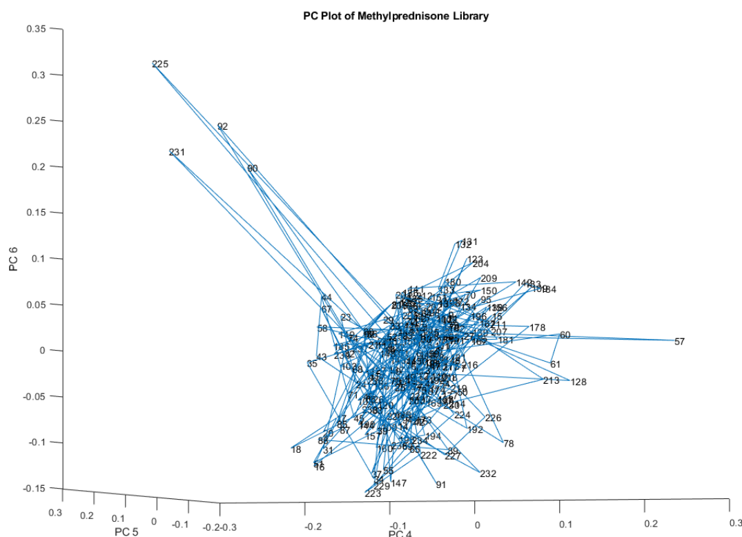
Figure 7. Scatterplot of principal components 4, 5, and 6 of the spectral library of 242 vials of methylprednisolone. These are the same spectra depicted in Figure 6 . The potential outliers in Figure 7 are vials 90, 92, 225 and 231.
