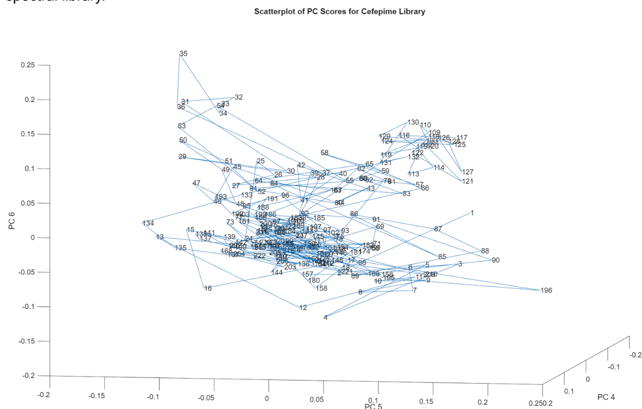
Figure 10. Scatterplot using PCs 4-6 of the scores of the spectral library of 222 cefepime vials
